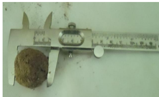
Figure 4: Pellet diameter measurement
