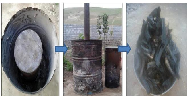
**Figure 1:** Biochar preparation via slow pyrolysis using a production oven
